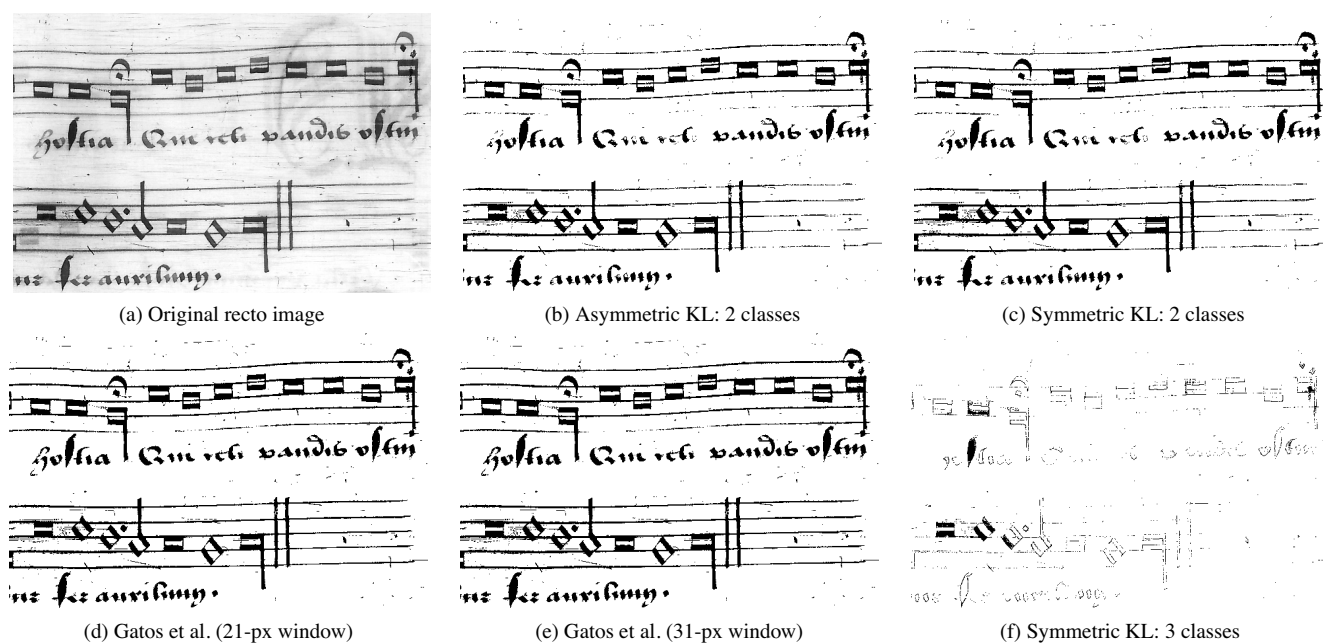
Figure 1: Binarization output from selected algorithms on a page of the Occo Codex.
